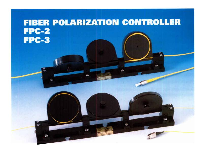
FIBER CONTROL INDUSTRIES polarization controller's unique user-friendly design utilizes stress-induced birefringence to alter and control the state-of-polarization of light in single-mode fibers. Each paddle acts as a fractional waveplate. Complete coverage of the Poincaré sphere and polarization control is provided by adjusting the angles of the paddles.
