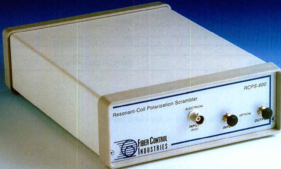
FIBER CONTROL INDUSTRIES Resonant-Coil Polarization Scrambler converts highly polarized light into light with a scrambled polarization by rapidly modulating the state-of-polarization — creating a time-varying birefringence within the fiber.
