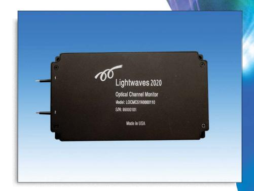
Lightwaves2020's innovative Optical Channel Monitor (OCM) is a very compact integrated module with multiple functions of optical channel monitor, optical performance monitor, optical wavelength meter, and DWDM spectrum analyzer. The OCM provides real-time and non-intrusive measurement and monitoring of optical channel power, wavelength and optical signal-to-noise ratio (OSNR).
