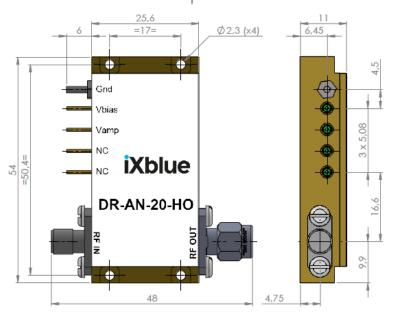
The heat-sinking of the module is necessary. It's user responsability to use an adequate heat-sink. Refer to page 5 for iXblue recommended heat-sink.
