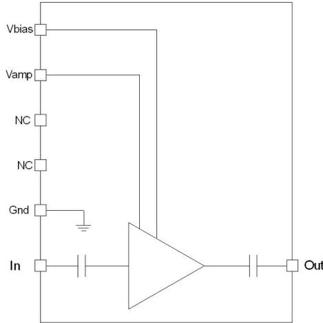
Mechanical Diagram and Pinout
