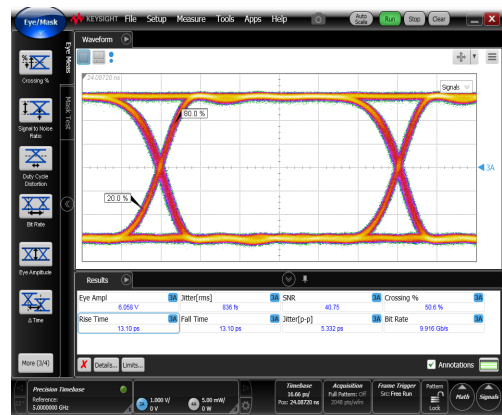
Output response Eye amplitude = 6 V pp
