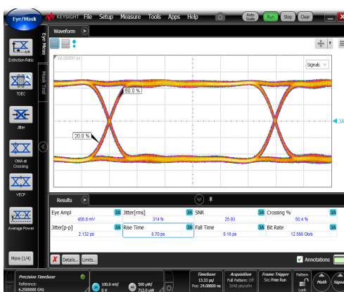
Input signal Eye amplitude = 0.45 V pp
