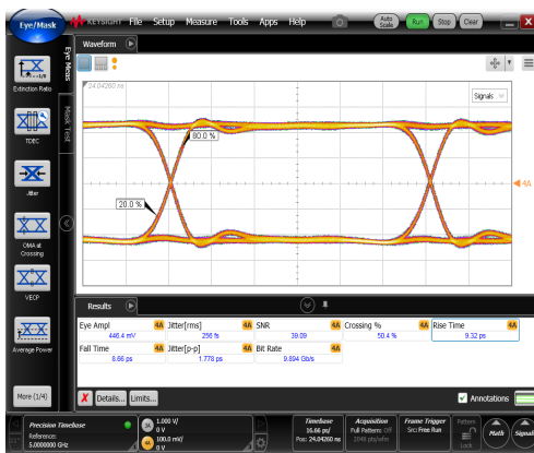
Input signal Eye amplitude = 0.45 V pp
