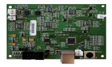
Unlike classical dither signal based bias controllers, MBC-AN do not superimpose any tone signal to the optical modulated signal. They are designed for application where such a tone signal is not desired and typically for analog applications where a high purity carrier is required. They are easy to implement, and are available as benchtop instruments and OEM boards.
