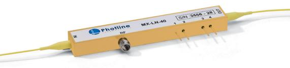
The MX-LN series are lithium niobate ( $\text{LiNbO}_3$ ) intensity modulators designed for optical communications at data rates up to 40 Gb/s.
