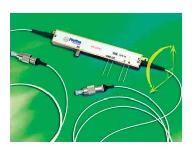
The Photline PS-LN Polarization Rotators are integrated optics waveguide devices that switch the polarization state of an input light between two linear orthogonal output states at frequencies up to 10 GHz. Practically, the output light is transmitted on either the fast or slow axis of the output polarization maintaining fiber of the component, operating then as a TE to TM converter.
