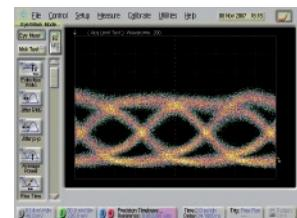
measured at +10 dBm optical input, PRBS 2<sup>7</sup>-1,
