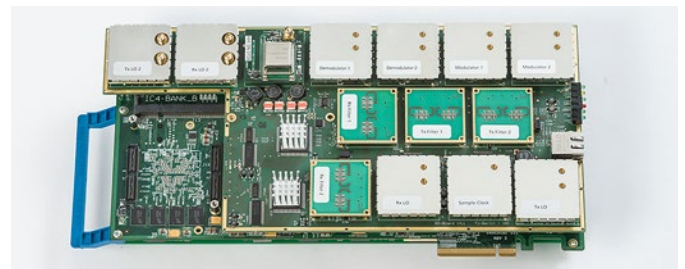
HIRATE transceiver board equipped with plug-on modules
