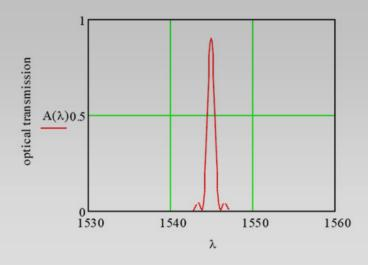
The Brimrose dynamic tunable bandpass filters are commonly used to dynamically select among different wavelength channels at the receiver end of dense WDM transmission systems.
