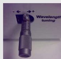
Fig. 5 Repeatable tuning through manual high resolution micrometer actuator.
