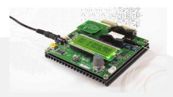
ULDC is a fully integrated laser diode controller with precise current and temperature setting. With a Zero Insertion Force (ZIF) adaptor, ULDC can be used with all 14 pin laser diodes.
