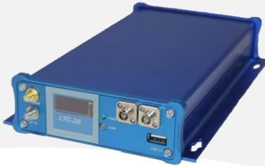
The Optilab LTC-20 is a high-performance Lightwave Transmitter Modulator that can be used with LRC-23-PA for RFoF conversion application.
