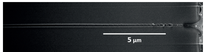
Laser drilling of a glass sample achieved with a CANUNDA-PULSE
