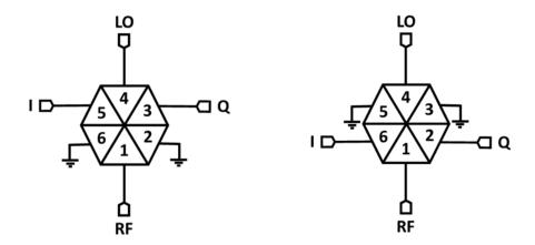
Choose one IF (I+ and Q+ or I- and Q-) and short the unused IF ports to ground Single ended operation allows for use of a DC IF signal
