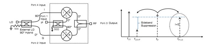
A band shifter is an unusual application for a mixer. Band shifters take an IF signal and shift it to a different band, generally to either avoid interference or for rebroadcast at a different frequency. For cases in which the desired band shift cannot be employed by using a standard up or down conversion scheme, an exotic input scheme is required.
