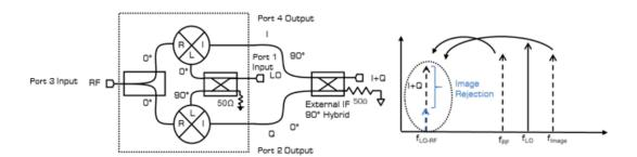
An image reject mixer is a mixer which rejects the down converted image frequency from the IF output. Image reject mixers are constructed using an external quadrature hybrid attached to the I and Q (i.e., IF) output ports. Using the external IF quadrature hybrid, one can select the whether the upper sideband or lower sideband signal is suppressed with respect to the LO signal.
