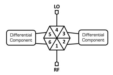
The mixer in its standard configuration is set up for use with differential IFs
