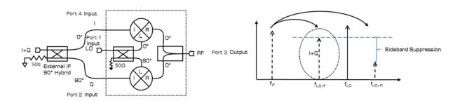
A single sideband mixer is a mixer which suppress the up converted image frequency from the RF output. Single sideband mixers are constructed using an external quadrature hybrid attached to the I and Q (i.e., IF) input ports. Using an external IF quadrature hybrid, one can select whether the upper sideband of the lower sideband signal is suppressed with respect to the LO signal.
