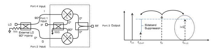
A band shifter is an unusual application for a mixer. Band shifters take an IF signal and shift it to a different band, generally to either avoid interference or for rebroadcast at a different frequency. For cases in which the desired band shift cannot be employed by using a standard up or down conversion scheme, an exotic input scheme is required.
