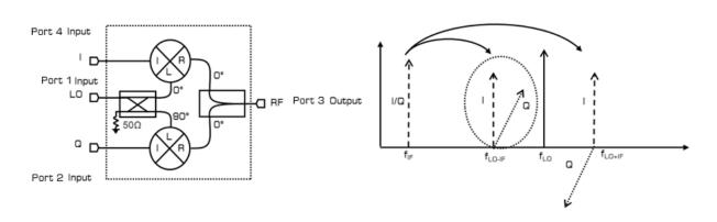
An up converter is a mixer application which takes a low frequency small signal IF input, and a high frequency large signal LO input and mixes the signal together to produce a high frequency RF output. The fundamental 1IFx1LO outputs present at the RF port are the  $f_{LO-IF}$  and  $f_{LO+RF}$  tones. An up conversion can select either the  $f_{LO-IF}$  or the  $f_{LO+IF}$  tones. The above illustration shows both up converted sidebands with either an I or Q port input signal.
