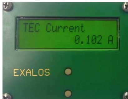
Fig. 10 Display-Board DIB5000 in display mode 4 (TEC current)
