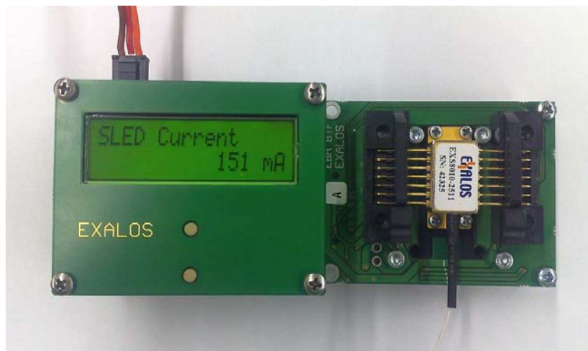
Fig. 4 Top view of an EBD5020 with an adapter board for 14-pin BTF modules
