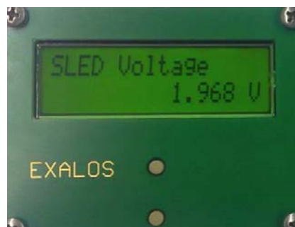
Fig. 8 Display-Board DIB5000 in display mode 2 (SLED forward voltage)
