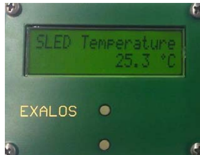
Fig. 9 Display-Board DIB5000 in display mode 3 (SLED temperature)
