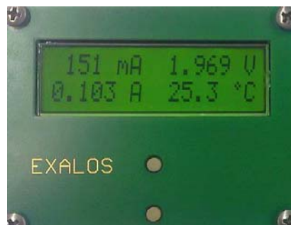
Fig. 11 Display-Board DIB5000 in display mode 0 (all four parameters)
