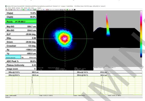
The WinCamD-IR-BB is supported by DataRay's full-featured, highly customizable, user-centric software which has no license fees, unlimited installations, and free software updates. The software supports M² measurements using our M2DU stages.
