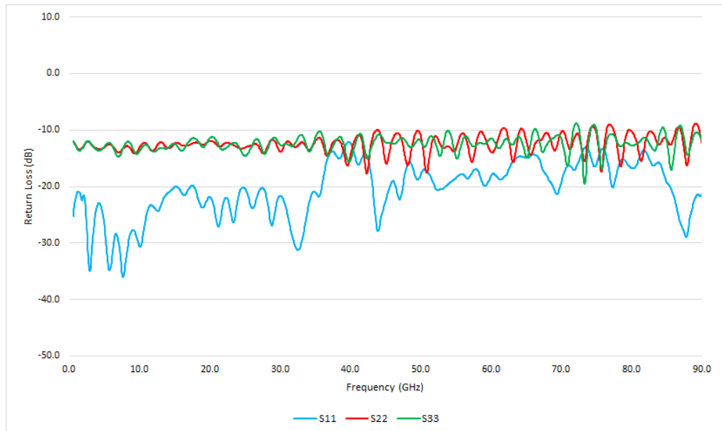
Figure 2: HL9408 Single-ended Return Loss
