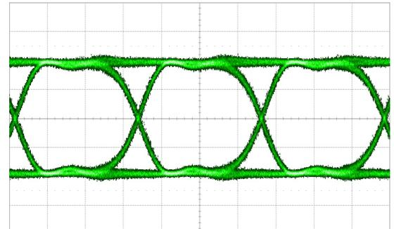
Figure 11: 12.5 Gbps PRBS31 pattern on Thru Out
