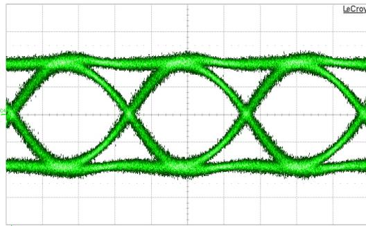
Figure 8: 28 Gbps PRBS31 pattern on Thru Out
