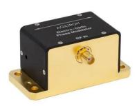
Our Free-space Electro-optic modulator (FEOM) in the resonant frequency is a electro-optical crystal based modulator which efficiently modify the phase, polarization or amplitude of a free-space laser. It is designed to be operated at a fixed frequency with narrow bandwidth. The resonance frequencies can be selected from 5 to 100 MHz. This resonant modulator can be conveniently driven by a standard laboratory function generator at the resonance frequency.
