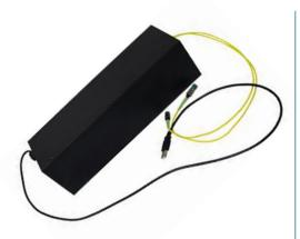
Agiltron's ITU Channel Tunable Filter selectively passes any wavelength channel on the ITU grid via a USB interface with a user friendly GUI. The configurations include up to 12 CWDM channels, 80 WDM channels with 100GHz spacing, and 96 channels with 50GHz spacing.
