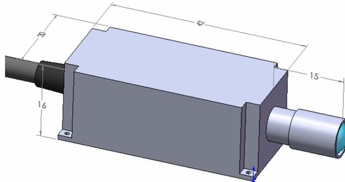
Typical 2000 mm isolator package dimension (only for 1 mm beam size)
