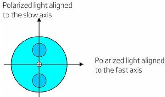
Note: The PM fiber and the connector key are aligned to the slow axis, fast axis is blocked.
