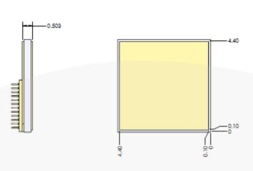
\*Chip length of COC-310 is 1mm. The diagram shown is for 2.5mm chip length.
