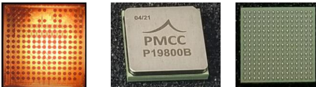
Figure 2. The ASIC chip and the BGA package.
