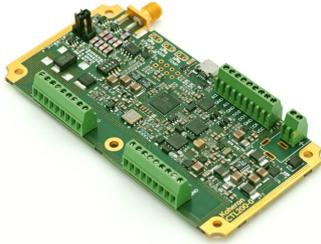
Koheron CTL200-0 is a digital low-noise laser diode driver combined with a TEC controller. It drives up to 600 mA laser current with a compliance voltage up to 3.2 V. It is the screw terminal version of the [CTL200 digital butterfly laser diode controller](#).
