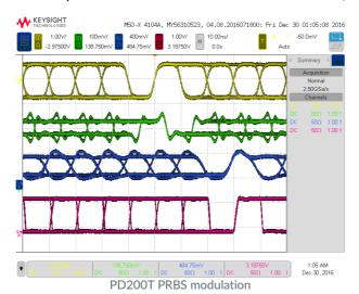
The 25 ns delay between the laser modulation (in orange) and the PD200T analog output (in blue) corresponds to the 5 m fiber between the laser and the PD200T.
