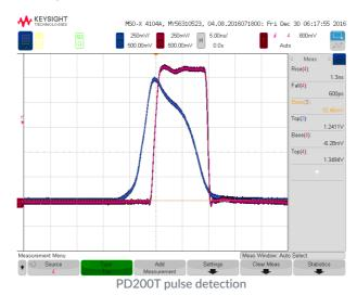
Propagation delay between the analog and the TTL output is about 2.5 ns. TTL rise and fall times (10 to 90 %) are 1.3 ns and 0.7 ns, respectively.
