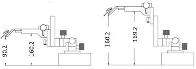
Total Coarse Height Adjustment: 70 mm Each Step: 5 mm
