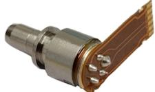
APX20D2-T03 is a receiver optical subassembly (ROSA) based on an Albis 28 Gbaud APD chip featuring large dynamic range and a high optical damage threshold of up to +5 dBm, and a multi-rate 25G burst-mode TIA offering high sensitivity with fast settling time.
