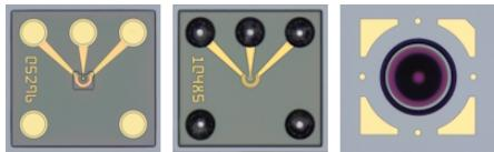
Ultra high-speed InGaAs/InP photodiode chip specifically designed for 200G PAM-4 applications (800GbE, 1.6TbE and 3.2Tbe). This chip features an integrated backside lens and offers excellent responsivity and high speed of response in the wavelength region from 1260 nm to 1620 nm.
