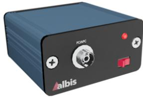
The PMX10A module is a self-contained, ready-to-use, 10 GHz multi-mode photodiode module for direct optical-to-electrical conversion of RF-modulated optical signals. The module is LiPo battery powered and USB-C chargeable with a conventional 5V phone charger.
