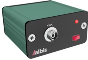
The PMY10A module is a self-contained, ready-to-use, 10 GHz single-mode photodiode module for direct optical-to-electrical conversion of RF-modulated optical signals. The module is LiPo battery powered and USB-C chargeable with a conventional 5V phone charger.
