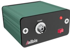
The PMY30A module is a self-contained, ready-to-use, 30 GHz single-mode photodiode module for direct optical-to-electrical conversion of RF-modulated optical signals. The module is LiPo battery powered and USB-C chargeable with a conventional 5V phone charger.
