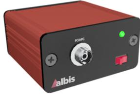
The PMZ40A-L module is a self-contained, ready-to-use, 40 GHz single-mode photodiode module for direct optical-to-electrical conversion of RF-modulated optical signals. The module is LiPo battery powered and USB-C chargeable with a conventional 5V phone charger.
