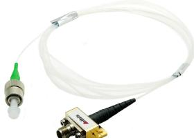
PQW10A-L is a long-wavelength, high speed microwave photodiode module designed for direct optical-to-electrical conversion of RF-modulated optical signals and provides a minimum bandwidth of 10 GHz. The optical input is supplied through a single-mode 9/125  $\mu$ m fiber pigtail. The RF output of the device is provided through a K-connector. The photodiode inside this module is a high performance Albis InGaAs p-i-n photodiode, designed to operate in the wavelength region from 1260 to 1620 nm.
