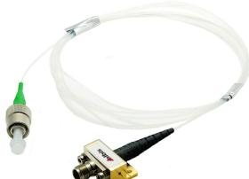
PQW10A-S is a short-wavelength, high speed photodiode module designed for direct optical-to-electrical conversion of RF-modulated optical signals and provides a minimum bandwidth of 10 GHz. The optical input is supplied through a multi-mode 50/125  $\mu$ m fiber pigtail. The RF output of the device is provided through a K-connector. The photodiode inside this module is a high performance Albis GaAs p-i-n photodiode, designed to operate in the wavelength region from 800 to 870 nm.
