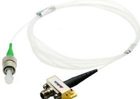
PQW10B-L is a high power, high-speed microwave photodiode module designed for direct optical-to-electrical conversion of RF-modulated optical signals around 10 GHz. The photodetector provides high responsivity of 0.85 A/W with a 3 dB bandwidth of 15 GHz and high linearity of up to 60 mA average photocurrent. It is designed to operate in the wavelength region from 1260 to 1620 nm.
