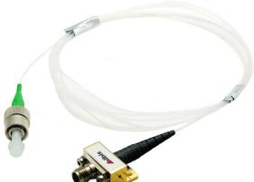
PQW20A-L is a high speed microwave photodiode module designed for direct optical-to-electrical conversion of RF-modulated optical signals and provides a minimum bandwidth of 20 GHz. The optical input is supplied through a single-mode 9/125 mm fiber pigtail. The RF output of the device is provided through a K-connector.
