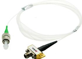
PQW20B-L is a high power microwave photodiode module designed for direct optical-to-electrical conversion of RF-modulated optical signals up to 20 GHz. The photodiode inside this module is a high power, high linearity Albis photodiode chip, designed to operate in the wavelength region from 1260 to 1620 nm. It offers a typical bandwidth of 22 GHz for photocurrents up to 50 mA, a responsivity of 0.8 A/W and high linearity of up to 50 mA average photocurrent.
