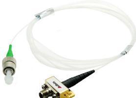
PQW20C-L is a high power, high-speed microwave photodiode module designed for direct optical-to-electrical conversion of RF-modulated optical signals up to the Ku-band. The photodiode provides high responsivity of 0.8 A/W with a 3dB bandwidth of 28 GHz. It enables high RF output power thanks to a linear response up to 13 mW average optical input power.
