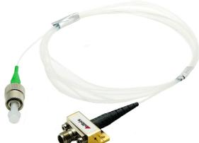
PQW30A-L is a high speed microwave photodiode module designed for direct optical-to-electrical conversion of RF-modulated optical signals and provides a minimum bandwidth of 25 GHz. The optical input is supplied through a single-mode 9/125 mm fiber pigtail. The RF output of the device is provided through a K-connector.
