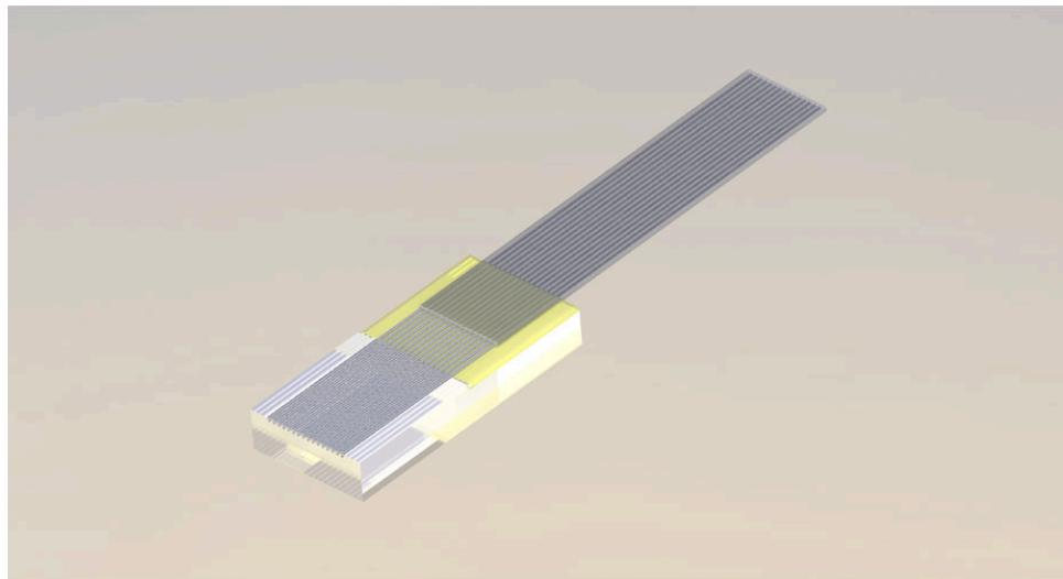
Lidless fiber array is an array with no glass lid pressing on the fibers. As for lidless fiber array, its fibers majorly populate in the grooves and are covered with only epoxy. In terms of its application, sealed application environment is better for this type of [V groove fiber array](#) (/products/linear-fiber-array/); A variant of lidless fiber array is lid-recessed fiber array, whose back part of fibers is the only area that is covered with lid.
