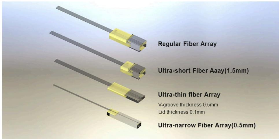
Ulrasmall fiber array specifically can be ultra short (2.5mm), ultra narrow(1mm) and ultra thin (0.6mm) to meet different applications. Ultra-short variant is an economical alternative to 90-degree FAUs used in surface fiber-to-chip coupling; Ultra-narrow and ultra-thin ones are normally needed in edge fiber-to-chip coupling with parallel optical architectures.
