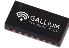
14 Pin 6x3 mm DFN Package
