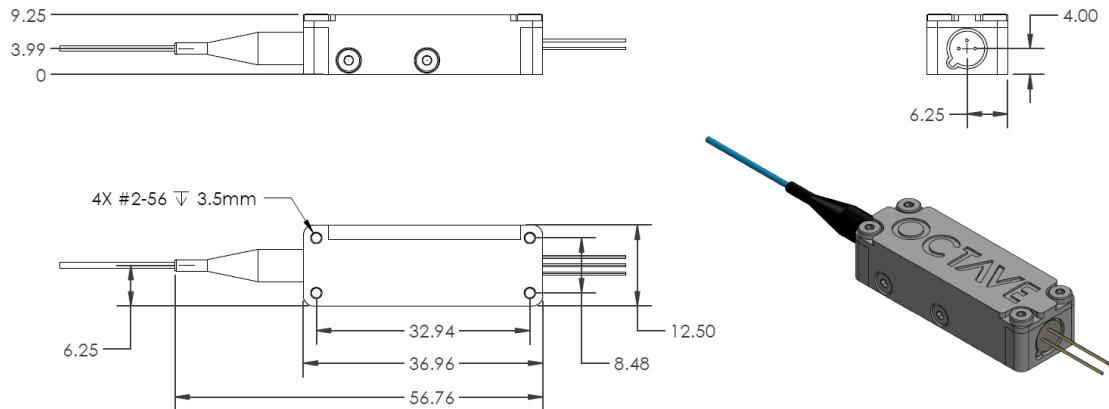
**COSMOO for high repetition rate:** For repetition rates higher than 2 GHz, the standard COSMO typically cannot be used. In such cases, we offer the COSMO with Optical output (COSMOO), which uses a lens to provide a collimated beam. The user can direct the beam to an appropriate high-speed photodetector to measure  $f_{CEO}$ .
