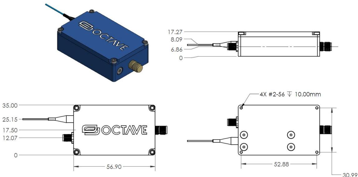
Dimensions are in millimeters. The SMA connector carries the CEO signal from detector. The 4-pin M5 connector provides inputs for detector power. The COSMO ships with an optional baseplate (not shown) to attach to standard optical tables.
