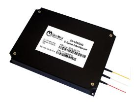
GouMax's UMI optical interleaver is a 3-port passive fiber-optic device that is used to separate Dense Wavelength-Division Multiplexing (DWDM) channels into two groups of signal streams (odd and even channels) in an interleaving way. GouMax's UMI optical interleaver uses an innovative design that features wide stopband and higher channel isolation. It provides the best solution to expand wavelength channel counts in DWDM system.
