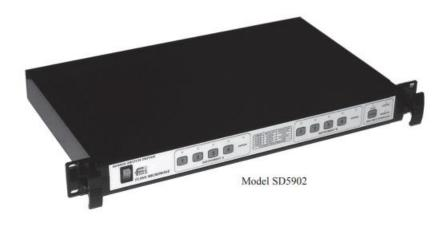
The Series SD5902 Waveguide Switch Driver is designed to control the Flann microwave range of Series 333-\*E Precision Waveguide Switches. It provides the interface between an IEEE 488 Bus (GPIB) or Universal Serial Bus (USB) and Precision Waveguide Switches and allows for manual operation with display of current status. The SD5902 will drive either a 2-channel or a 3-channel switch without the need to reconfigure.
